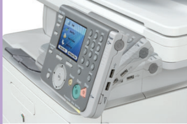
Tilt Control Panel
