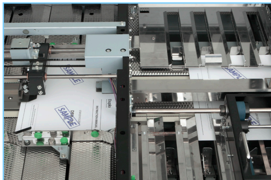
Two jogging areas jog each subset prior to scoring and folding to ensure the precise alignment of the sheets.
