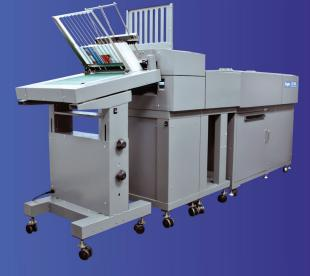
Incorporating an in-line knife folder with a DC-series finisher.
