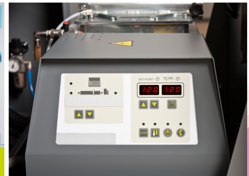
Built-in PUR tank and meter
