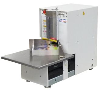
The RC-7 is a heavy-duty electric corner rounding machine with the capability to handle up to a 2.75" (70 mm) stack at a time. It features a detachable pressing bar, which helps secure documents for the cutting process and detaches for easy replacement of knives. Engineered for simple operation, the RC-7 can be operated by either a foot pedal or manual hand switch.
