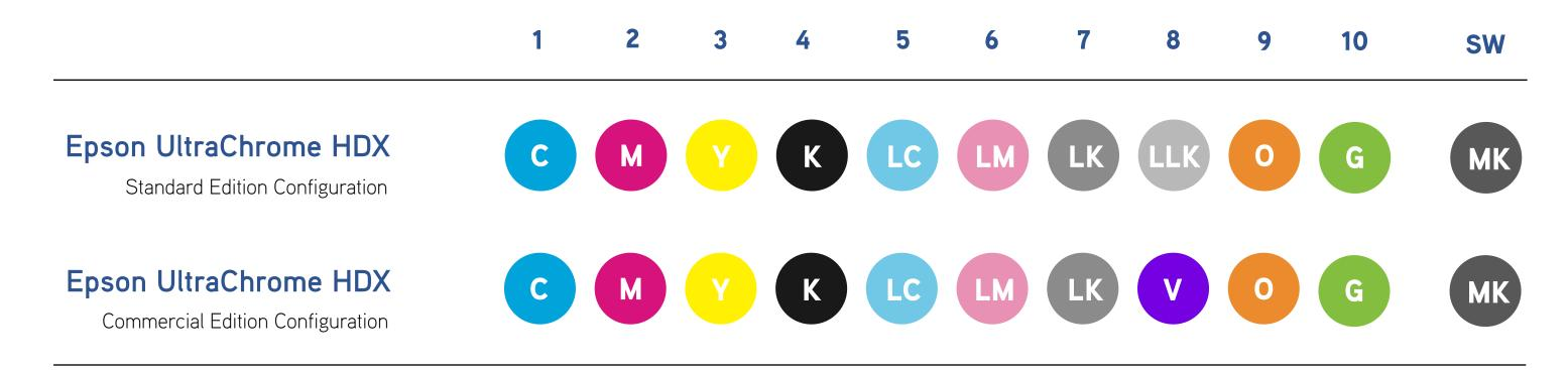
Due to the removal of the extra LLK ink, the UltraChrome HDX Commercial Edition Configuration is not intended for photo applications.
