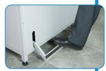
Foot pedal pre-clamp holds paper to check alignment prior to cutting
