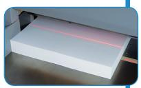
LED Cutting Line shows exactly where the blade will cut
