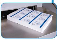
Low-friction work table and extra-large side tables help operators process large and/or heavy paper stacks with ease
