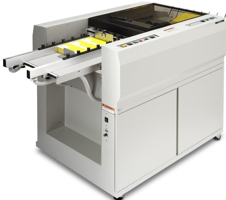
The FD 4400 industrial strength cut-sheet burster is specifically designed to process Check21 IRD's and other documents printed on perforated cut sheets. The FD 4400 sets the benchmark as the only high-volume cut-sheet burster capable of processing up to 30,000 forms per hour and up to one million forms (input) per month. The FD 4400 utilizes a bottom-feed air system, allowing operators to continually load forms to maximize efficiency and throughput.
