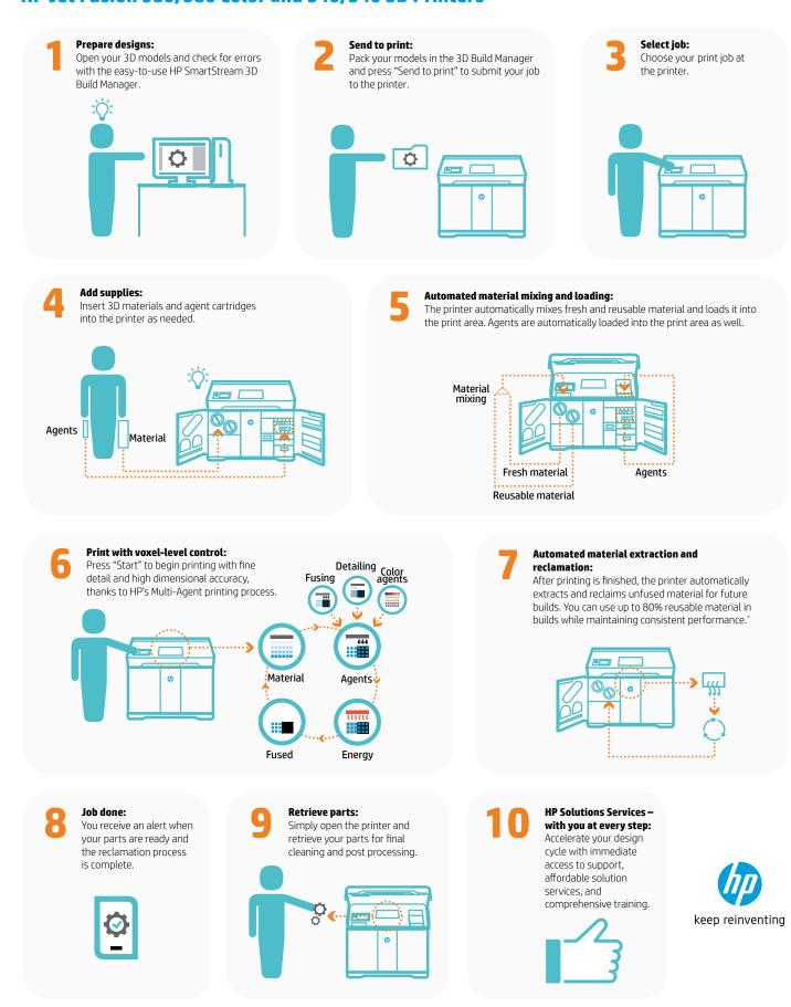
\*HP Jet Fusion 3D printing solutions using HP 3D High Reusability CB PA 12 provide 80% post-production surplus powder reusability, producing functional parts batch after batch.
