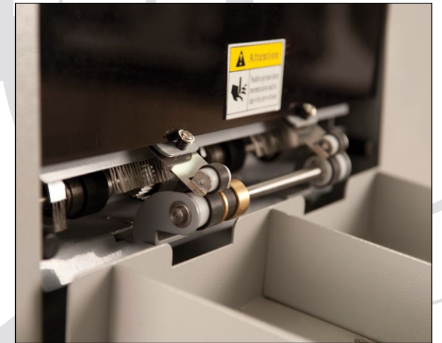
Long lasting slitter wheels and cross cutter blade
