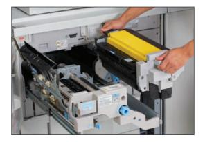
All systems feature Trained Customer Replaceable Units (TCRUs), which trained operators can replace quickly to maximize uptime without calling for service.
