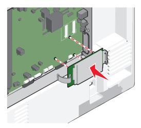
**b** Use the two provided screws to attach the printer hard disk mounting bracket.
