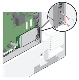
c Insert the plug of the printer hard disk interface cable into the receptacle of the system board.Note: The plugs and receptacles are color-coded.
