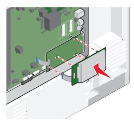
d Insert the plug of the printer hard disk interface cable into the receptacle of the ISP.Note: The plugs and receptacles are color-coded.
