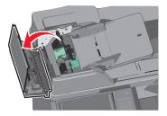
**4** Remove the pick roller assembly.
