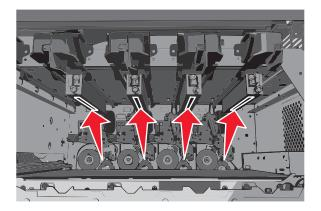
4 Clean the lenses using compressed air.
