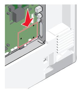
**4** Remove the printer hard disk.
