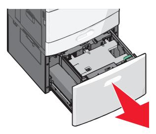
**2** Adjust the width guide as necessary.
