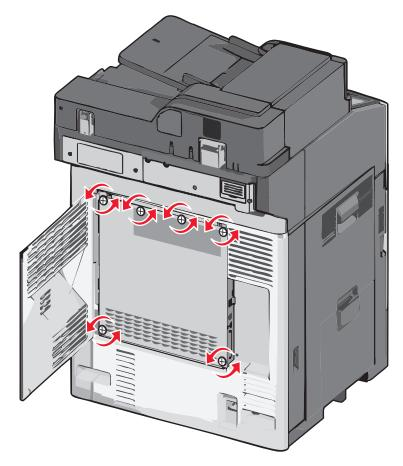
**b** Shift the metal panel to the left to disengage the hooks, then pull forward to remove it.
