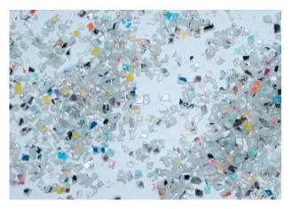
**SMALL PARTICLE SIZE** Each CD or DVD is shredded into approximately 1,200 particles, 3/32" x 5/32" in size. The photo shows actual particle dimensions.
