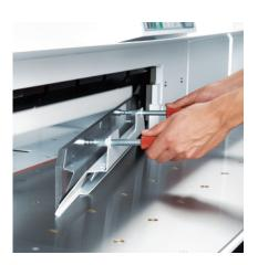
SAFE BLADE CHANGES Blade changes can be made without removing the machine covers. The handy blade changing device covers the cutting edge of blade.
