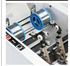
Magnetic stitching heads feature one-step threading for quick and easy set-up.
