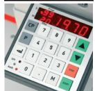
The "EP" back gauge control module stores 99 programs and frequently used measurements.
