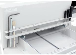
DROP-IN TOOL HOLDER Convenient, drop-in tool holder is located on the rear of the machine and keeps all tools necessary for routing maintenance (including blade changes) within easy reach.
