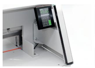
IR LIGHT BEAM SAFETY CURTAIN Safe and efficient cutting is ensured by the front table IR light beam safety curtain.
