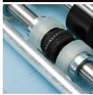
Built-in perforating wheel is easily engaged for in-line perfing
