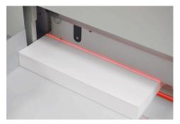
LED cut line allows operators to make fine adjustments and see exactly where the blade will cut
