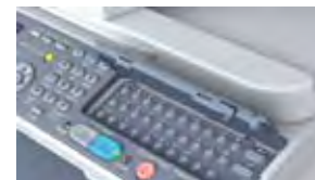
1-Touch key panel flips up for QWERTY keyboard
