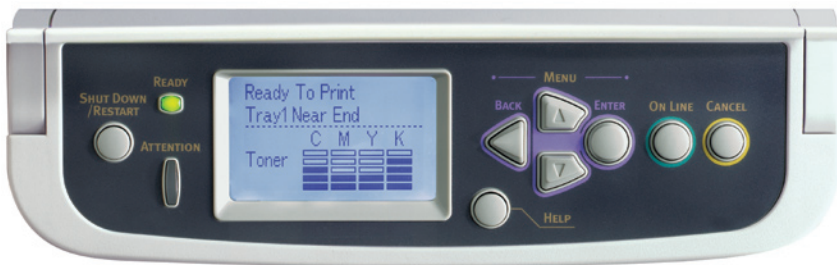
The easy-to-read operator panel of the C9650 Series tilts up for user convenience, and displays current status of the printer. A built-in toner gauge indicates the remaining life of each toner cartridge.
