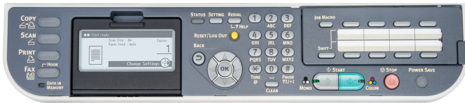
MPS4700mb MFP Operator Panel (backlit LCD display tilts up as much as 90°)
