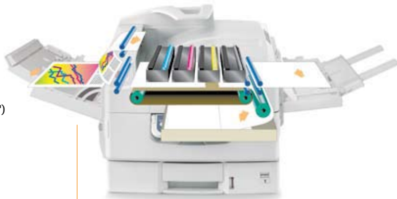
Single Pass Color™ technology and straight-through paper path handles thick paper stock and banner sheets.
