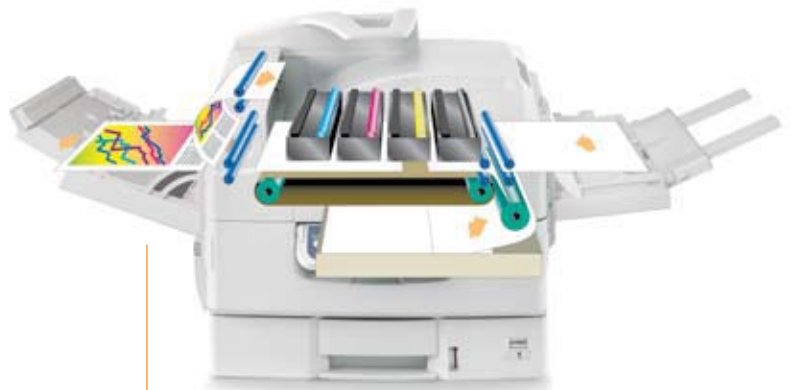
Single Pass Color™ technology and straight-through paper path handle thick paper stock and banner sheets.
