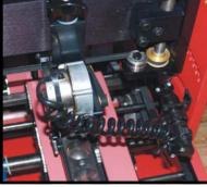
Dynamic Rotation Technology separators that can be removed and slid to the position needed.
