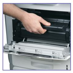
The all-in-one (AIO) print cartridge is ideal for users without technical training. Easily accessible within seconds simply by opening the front cover, this convenient feature restores output to "like-new" image quality.
