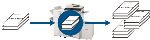
Multi-page original is scanned... stored on hard disk in proper page order... and stacked offset (or print data sent from PC)
